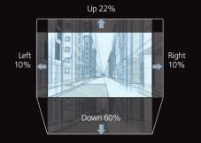
\* This figure shows the lens shift range for the projector with the optional lens SD-903 at the ceiling mounting posi
