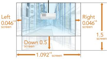
\*4 0.044 screen to left or right (Total 1.088 screen) for CP-WU5506M. \*This figure is not drawn to scale.
