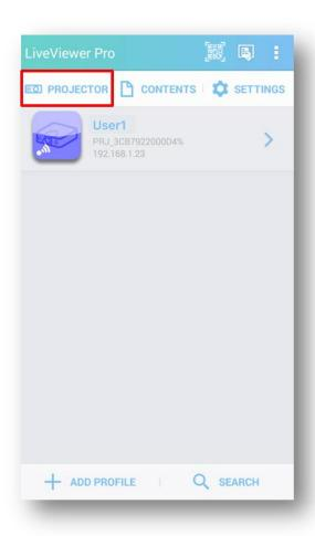
On the projector tab, you can set the connection between the smartphone and the projector. "Profile list" is opened when in case profiles are registered when LiveViewer Pro is started up. If the profile is not registered, "Discovery List" is opened.
